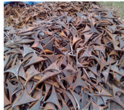
废钢废铁 (剪切后) Steel Scrap ( After Shear)
