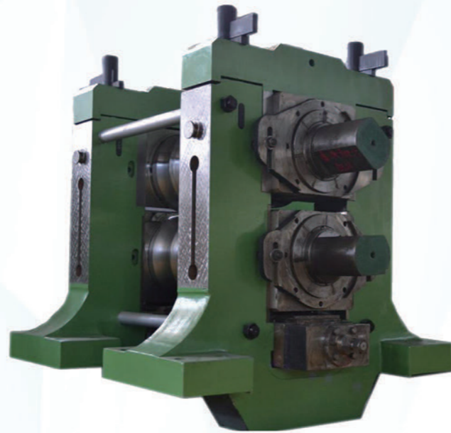
二棍涡轮蜗杆下调整轧机 2-Hi Roller-Worm Gear Bottom Regulation
