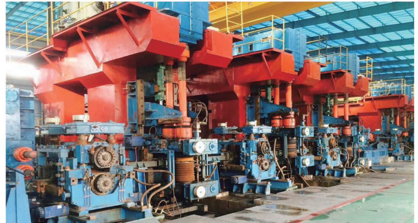
平立交替短应力轧机列组 H-V Alternating Short Stress Rolling Mill Production Line
