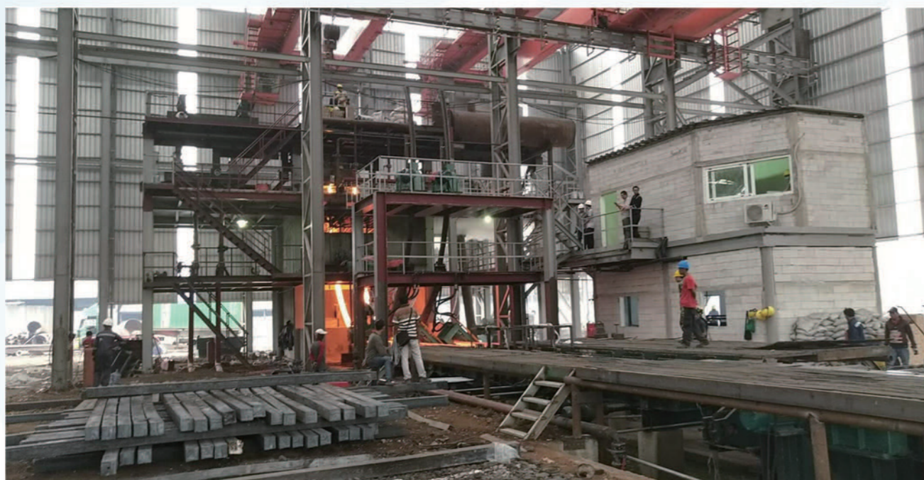
R6米-两机两流弧形连铸机 R6m-2 Strands Countnuous Casting machine
