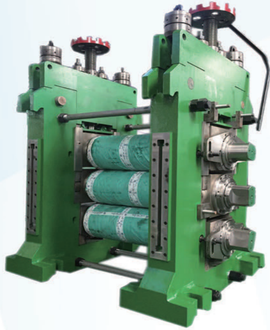
三辊上调整轧机 3-Hi Roller-Separate Locking Upper Regulation
