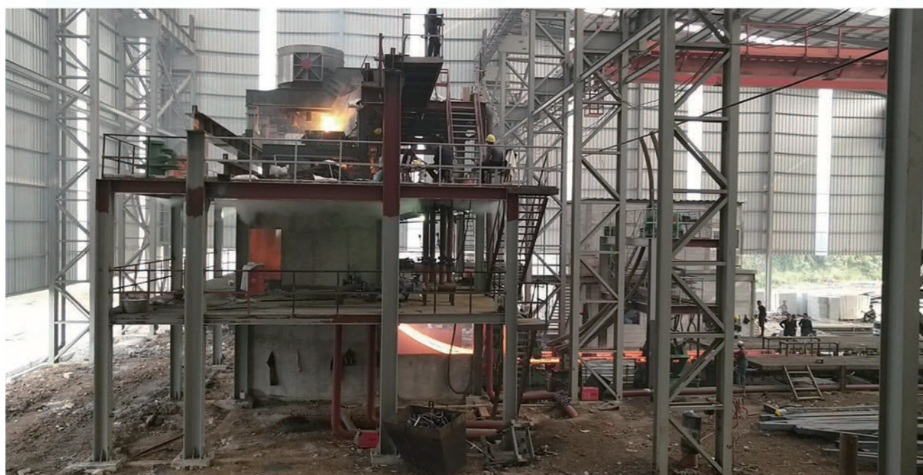
R6米-130方-150方 钢坯连铸机 R6m-Billet 130x130mm-150x150mm Countnuous Casting machine
