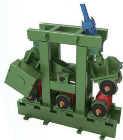
弧形热刚坯-拉矫机 Ithdrawal&Straightening Machine
